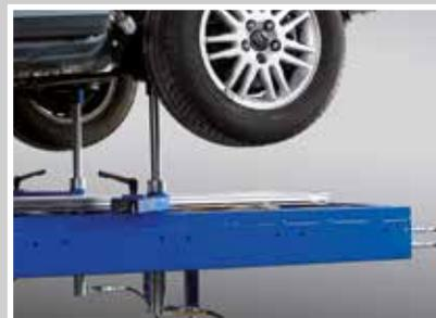
**Efficient vehicle mounting** with hydraulic pillar jacks
