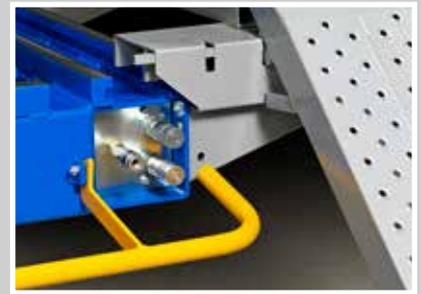
**Integrated** multi-functional power unit for hydraulics, lift, pulling towers and air tools
