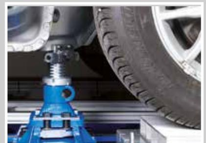
**Effective holding and clamping** with no need for dedicated, vehicle specific fixtures when using the EVO 1, 2 & 3 holding and anchoring system
