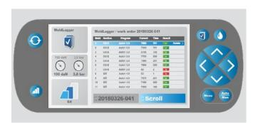
The **CTR 9** records weld data and generates reports during the repair process. Print the report to testify to the quality of the welding and increase the trust in your body shop.
